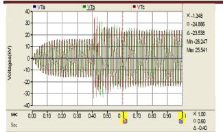
**Fig. 3** 13.8kV phase voltages of unloaded tertiary winding of 502 MVA Transformer with load rejection at 110kV Substation. **Table 3**: Summary of Temporary overvoltages at Tertiary (13.8kV
